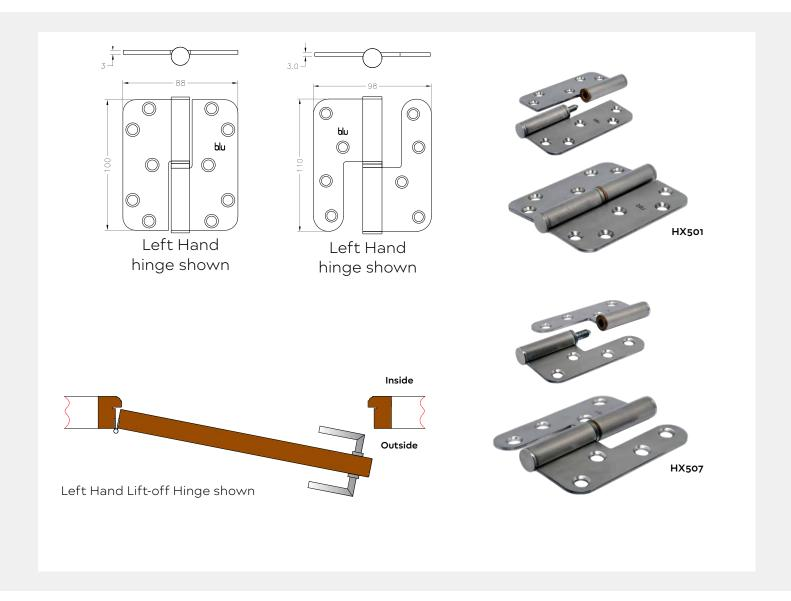
HX501 and HX507 are handed products - the hinge leaf with the pin is fitted to the frame, the other half with the receiving hole is fitted to the door, allowing the door to be lifted off.
